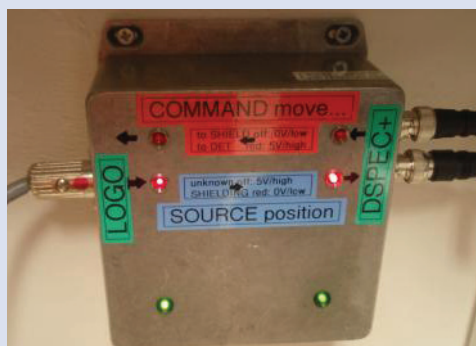
Figure 14. Automated system for energy recalibration of CTBT detectors at ATLO3, Seibersdorf, Austria.
