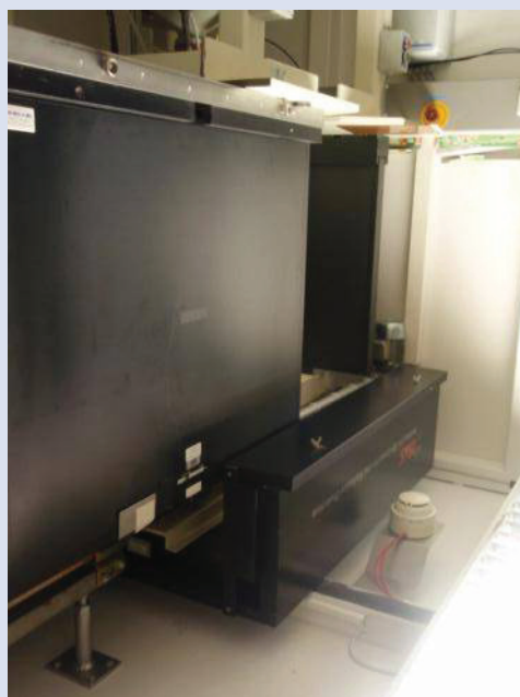
Figure 15. Cosmic veto system for CTBT detector at ATLO3, seibersdorf, Austria.
