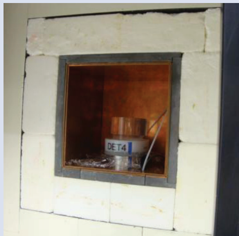
Figure 13. Clean lead, copper and boron adsorbers in CTBT detector at ATLO3, Seibersdorf, Austria.
