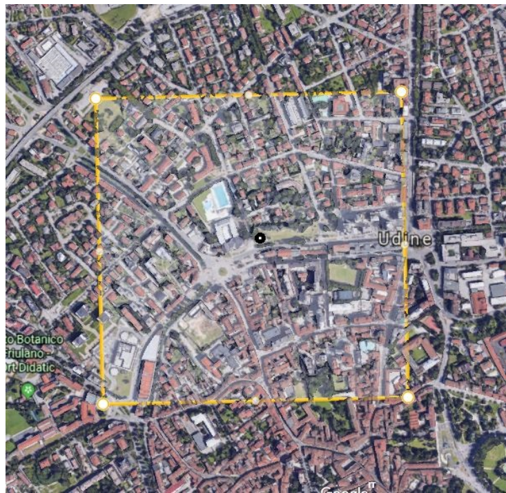
Figure 4.4: The chosen domain. The white dot is the position of the air quality station; in UTM33 coordinates (363109, 5103452)m.
